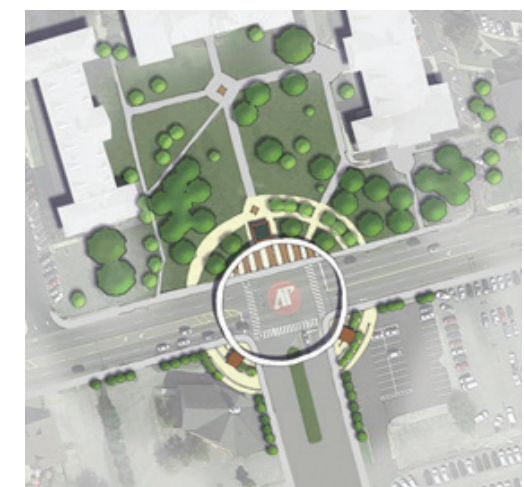
Elevated Circular Crosswalks
