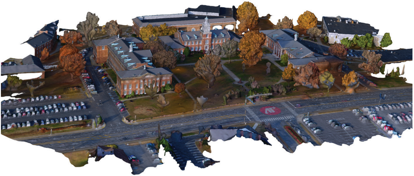
Using a consumer-grade drone and specialized software, Doug Catellier is able to render a fully intractable 3D model of Austin Peay State University's Clarksville campus out of hundreds of photos taken using the drone's onboard camera.
